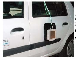
...Through a last generation license plate recognition, embarked on a vehicle
